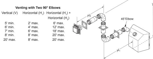
Figure 17 - Horizontal Termination Configuration for Venting Using Two 90° Elbows
